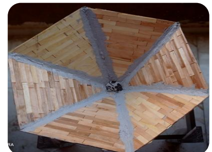
Figure (25) shows the internal of the prototype after covering by Kempoxy 150.
