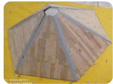
Figure (23) shows the faces after putting them together by PU sealant.
