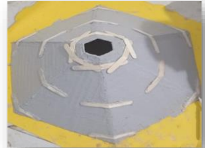
Figure (24) shows the supported prototype after covering by PU sealant and Kempoxy 150.
